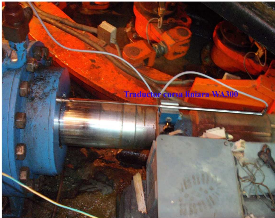
Fig. 10 Measuring scheme of the actuator piston linear stroke
