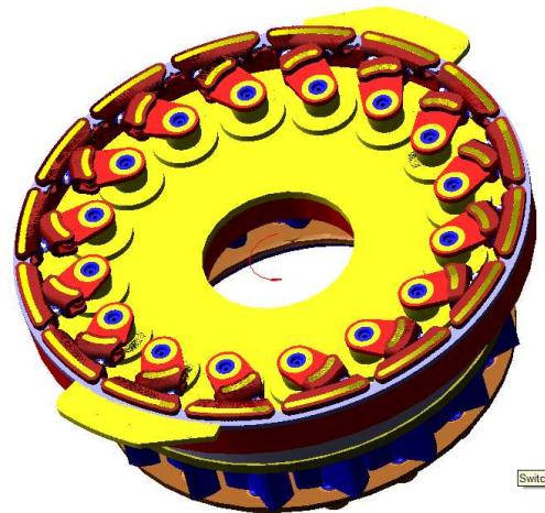
Fig. 4 3D Model of the wicket gate mechanism, imported in ADAMS, C pair, 3D simulation.
