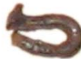
Fig. 20. Nail, access pillar of the porch, side V Dragomirești northern tip of the wooden church, Maramures County, dated 1722, displaced in the 1936 MNS "DG" total length of 18 mm, 0.92 mm diameter
