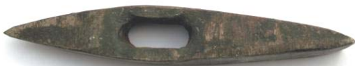
Fig. 14. Hardware tool (for cutting and punching); 4/4 19 th century; L = 180 mm; l = 27 mm
