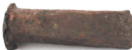
Fig. 10. Short chisel, 1/4 19 th century, L = 124 mm; l lamă = 30 mm; D = 35 mm
