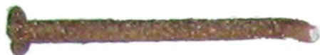
Fig. 21. Nail, porch, N side, western wood Church Timișeni, Gorj County, dated 1773, displaced in the 2002 MNS "DG" total length 30 mm, 1.4 mm diameter
