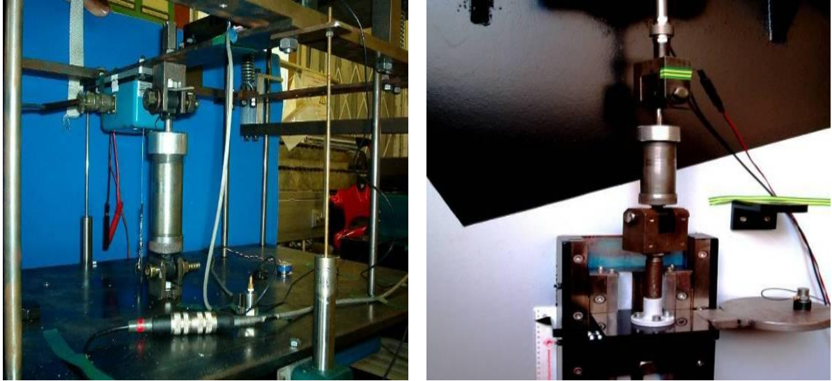
Fig.4 – The fixation module of the MR damper and of the acceleration transducers, speed, movement and testing of the MR damper model testing on the IMS stand
