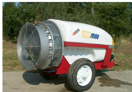
Fig. 2 - Sprinkling machine for vineyard, orchard, VUR 1000
