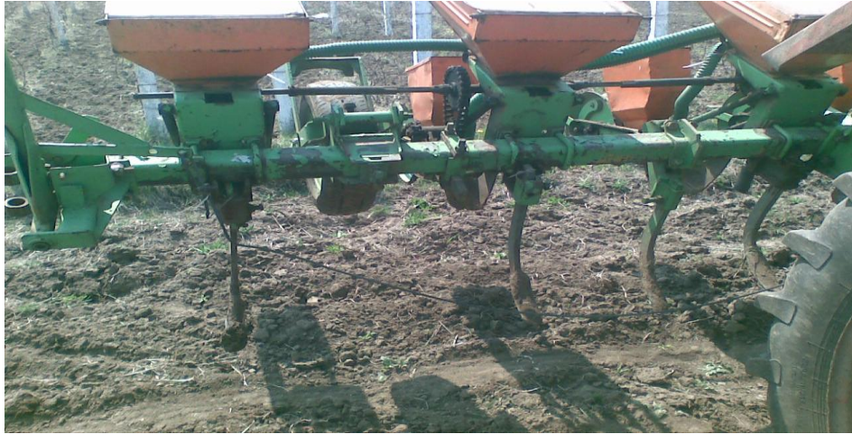
Fig.2. Sowing machine for weed plants – improved variant
