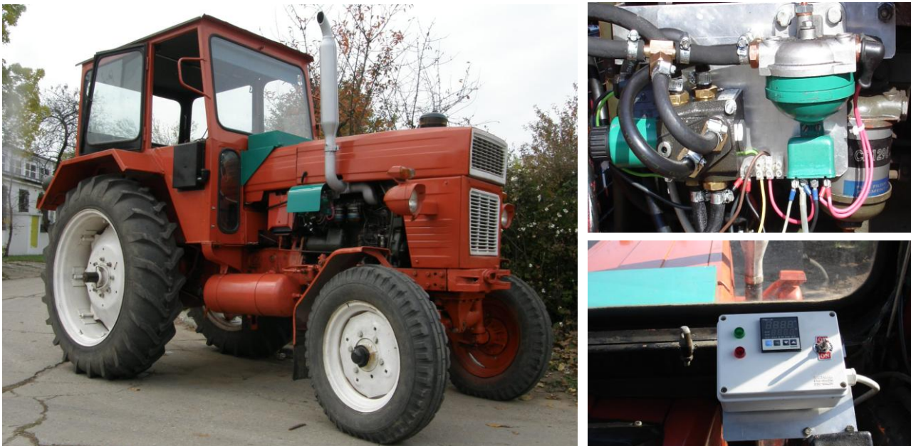
Fig. 2. Equipping the U650M tractor with a Diesel engine vegetable oil pre-heating system
