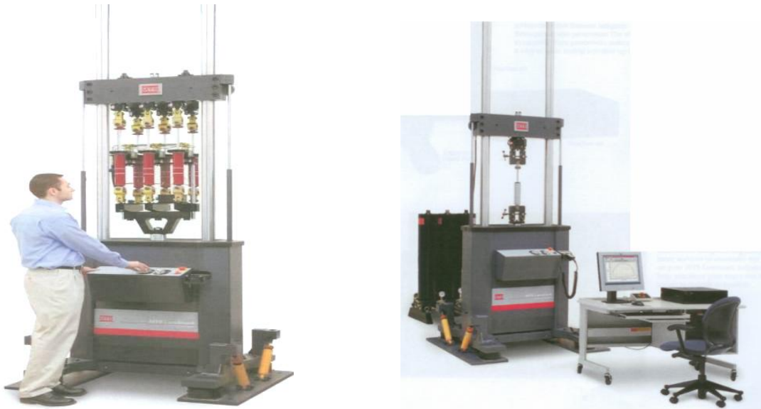
Fig. 6 – Stand for damper test produced by MTS Landmark
