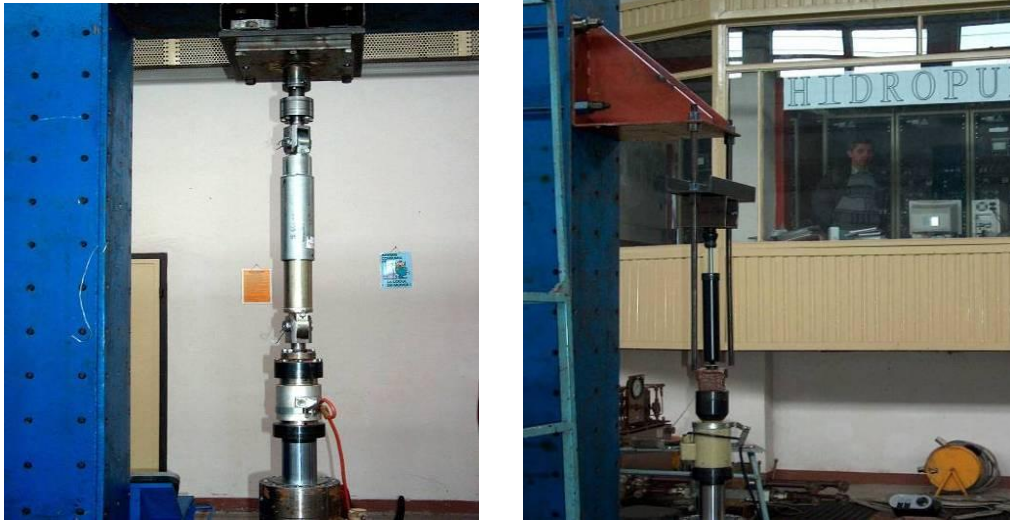
Fig. 2 – Stand for damper testing – INMA – Bucharest
