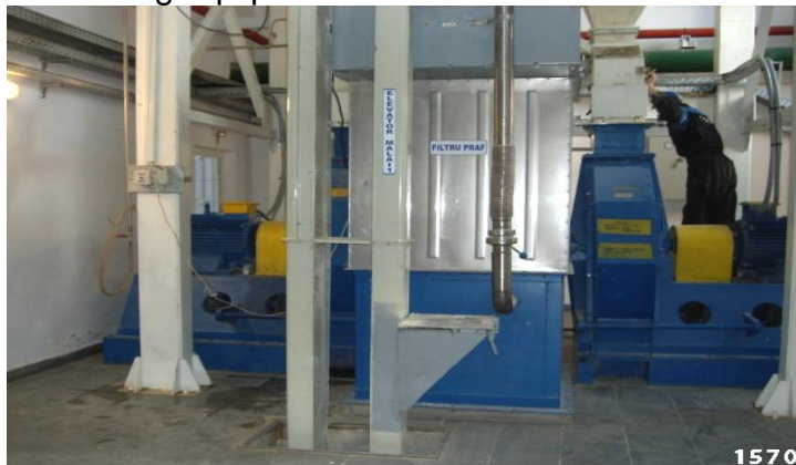
Pic.3 – Milling equipment with two hammer-mills
